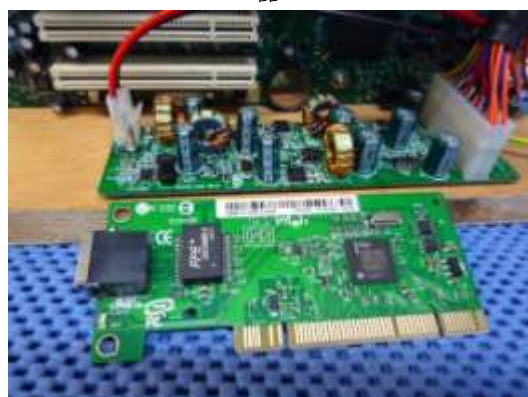
图 4 添置 Gigabit Lan Card 和 12V DC Power Supply
